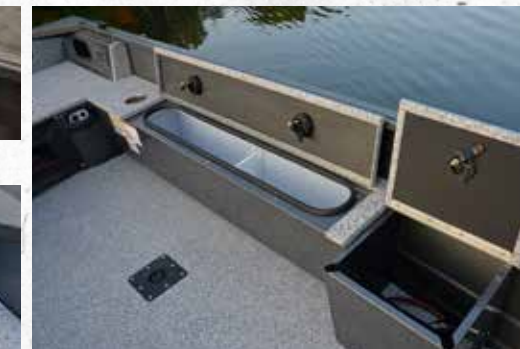
Outfitter 160 port side livewell and battery box
